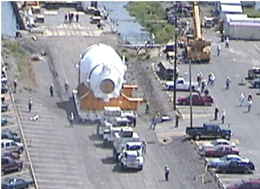
Barge offload and steam generator transport. Arkansas Nuclear one
