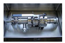
Tool to take a gas sample for radiolysis (developed for spent fuel containers type TN 17T)
